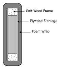
For testing purposes a typical panel construction consists of a soft wood frame with plywood frontage covered in 2mm HR foam. The panel fabric to be tested is then clipped around the panel and positioned the test rig. The base is constructed of chipboard covered in laminate to simulate a desk top. The vertical surface test also includes a watersoak procedure for the fabric.
