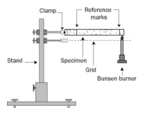
For materials which melt or shrink away from the heat source, after flame, non-propagation of flame and burning/non burning droplets are observed. Rate of flame spread is also measured if the material does not achieve M3.
