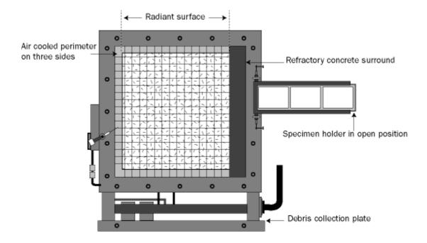
The test equipment consists of a vertically mounted radiation panel, supplied with a gas-air mixture, together with a specimen holder and pilot flame arrangement mounted to one side. The specimen holder swivels so that it is located at 900 to the face of the radiation panel during the test.
