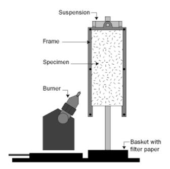
The fabric specimen is suspended vertically and a 20mm high flame is applied for 15 seconds to both the fabric surface and edge. Reference lines are marked on the specimen, which achieves B2 classification if the tip of the flame does not reach the reference marks within 20 seconds on any sample. 5 samples are tested with filter paper being placed below each to determine the production of flaming droplets.
