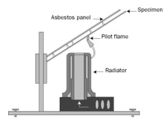
The sample is placed face down on the test rig at an angle of 30o above an electric radiator which gives out heat. A small butane gas pilot flame is applied directly to the fabric surface at 20 seconds into the test, held in position for 5 seconds then withdrawn. The flame is applied again at 45 seconds and subsequently every 30 seconds for the duration of the 5 minute test. If any flaming continues after 5 minutes, the test is continued until the specimen extinguishes completely.
