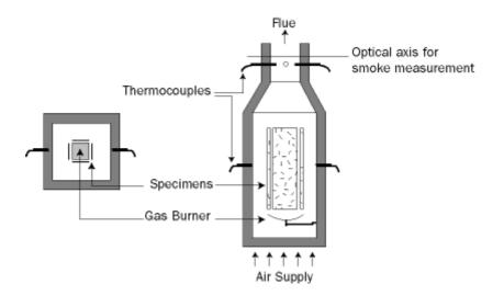
In evaluating the test, smoke gas temperature and the mean residual length of the sample are taken into account (residual length is the part of the specimen which has escaped burning). In order to be classified as B1, the tested fabric must show:
