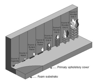
Of the eight ignition sources, the most frequently used are Ignition Source 0 (cigarette), Ignition Source 1 (butane flame/simulated match) and Ignition Source 5 (Crib 5). Moving up the ignition source scale, the heat intensity roughly doubles as compared to that of its predecessor.
