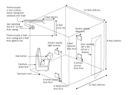
The ignition source is a square gas burner placed in the furniture seat, 2" from the back and 1" above the base. The flame exposure time is 80 seconds.
