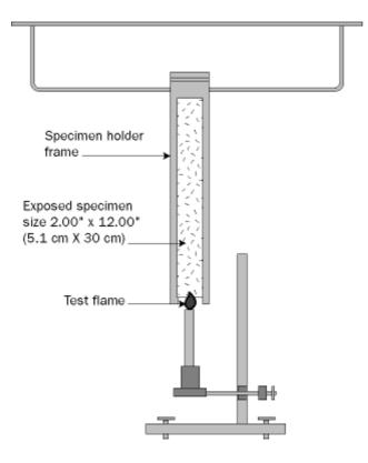
The fabric specimen is suspended vertically and subjected to a 1.5" methane flame for 12 seconds. Afterflame, drip burn and char length are monitored.
